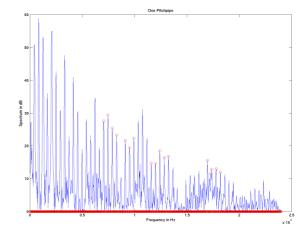
Figure 1. Spectrum of a piece of pitchpipe signal. Components that cause excess masking are marked with circles on top of them.
