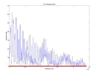
Figure 2. Spectrum of a piece of two-pitchpipe-mixed signal. Components that cause excess masking are marked with circles on top of them.
