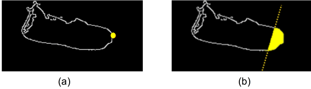
Figure 10: Finding the front point. (a) Original method. (b) Finding a small region in the front of the contour.
