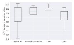
**Fig. 3**: Boxplot of the distribution of DTW distances between normalized MFCCs extracted from solo singing audio and corresponding original mixed audio, extracted vocals using various audio source separation.
