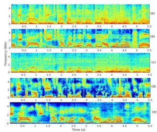
**Fig. 2**: Comparison of spectrograms for different audio source separation methods for "this afternoon" song from Hansen's dataset, (a) original mixed audio, (b) original clean audio, extracted vocal using (c) harmonic/percussive, (d) CNN based, (e) U-Net based audio source separation method.
